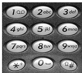
Fig. 1. A mobile phone keypad following the ITU-T E.161 mapping of numeric keys to alphabetic symbols. Non-standard mappings exist for key 1 (symbols such as punctuation), key 0 (spaces), and the * and # keys – one of which is usually assigned to “cycle”
